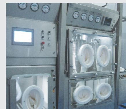
Integration isolation system with filtration, drying, weighing and filling process
