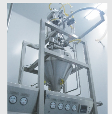
Integration isolation system with filtration, drying, weighing and filling process
